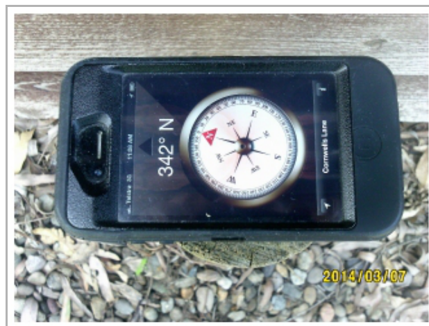
Figure 1: Using an iPhone to Determine Building Alignment
