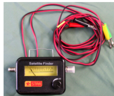
Figure 13: Completed, Modified SF-95 Satellite Finder Meter
