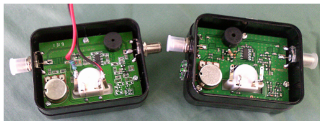
Figure 2: PCB Layout for the Sample Satellite Finders (SF-95 on left)
